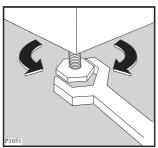
Any necessary adjustment can be made with a spanner. Accurate levelling prevents vibration, noise and displacement of the machine during operation.
